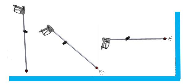
When starting to spray, keep the gun in upright position with nozzle facing down. Press the trigger and the nozzle will start rotating. You can now start moving to horizontal position at area to be blasted.
