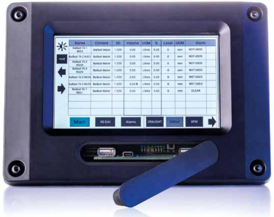
**Configurable remote tank level display.**
